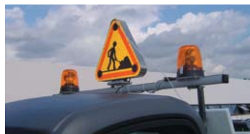
Roadsign bar (with 2 beacon lights)
